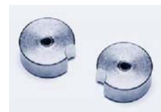
Sensor test “studs”
