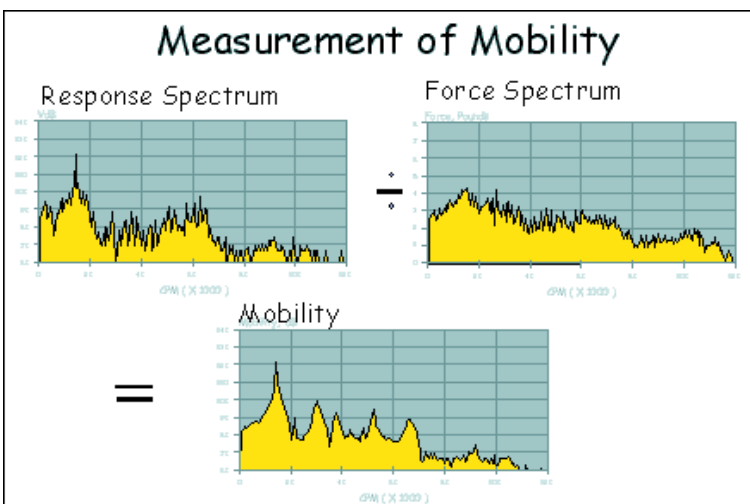
Figure 3 - We will need to enter the vibration levels at every frequency in a range and our mobility and force will look like spectra.
